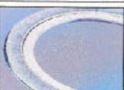
**Style RIR** - Built-in metal ring acts as a compression stop and fills the annular space between flange inner and the inside diameter of the gasket. Designed to prevent accumulation of scale, reduce turbulent flow of process fluids and minimize erosion at flange faces. Suitable for male and female pipe flanges.
