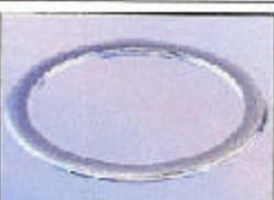
**Style R** - Basic construction type. Inner and outer elements are reinforced with several layers of metal without filler to give greater stability and better compression and sealing characteristics. Suitable for tongue and groove male and female or grooved to flat face flange assemblies.
