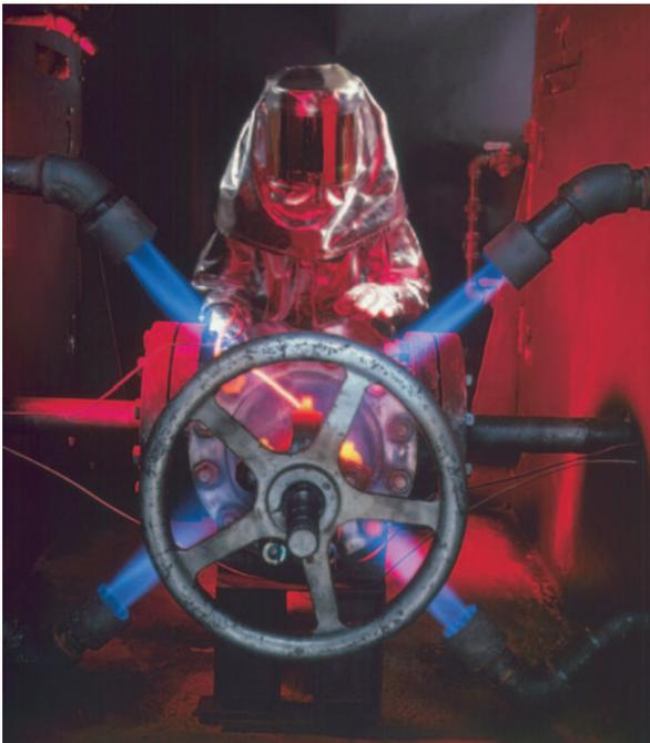
At the Garlock on-site fire test facility, valves and sealing materials have been tested for functionality in the most extreme applications. G-9900, 9800, 9850, ST-706 and IFG® 5500 meet these stringent fire test standards.
